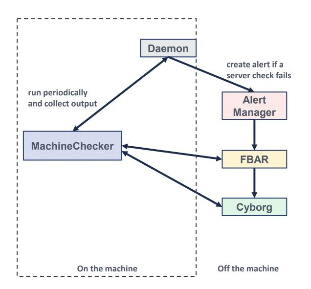
Failure Detection – MachineChecker
