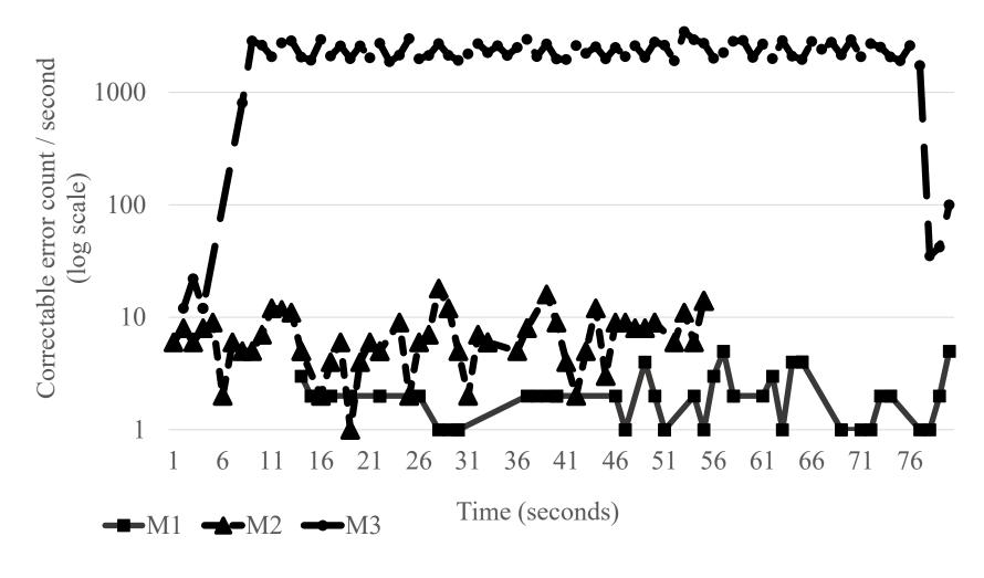
Observation 1: System Management Interrupts (SMI) cause the machines to stall for hundreds of milli-seconds based on the logging handler implementation. This is measurable performance impact to report corrected errors.
